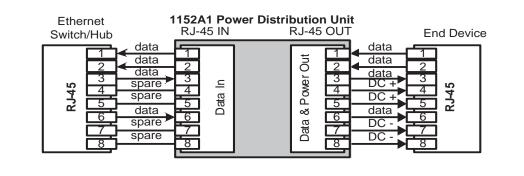
For Data-In ports connect the Ethernet cable leading from the Ethernet Switch/Hub to the Data port. For Data & Power Out ports connect the Ethernet cable leading to the telephone or other end device to the corresponding Data & Power port.
